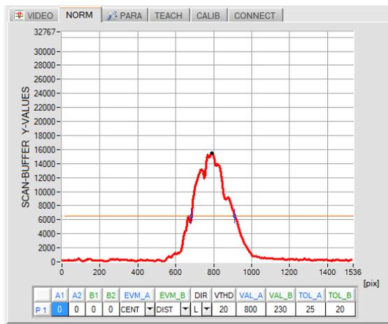
The picture opposite shows a typical picture of a spray recording. Above the X axis (pixels of the line sensor) the spray density distribution is visible as a red curve. Using an adjustable search threshold THD [%] (orange horizontal line), intersection points (edges) can be derived from the density profile. A black cursor indicates the position / height of the density maxima.
