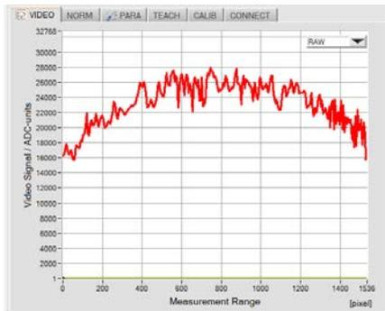
The laser power is adjusted in the VIDEO tab.
