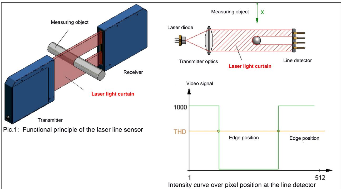
Pic.1: Functional principle of the laser line sensor
